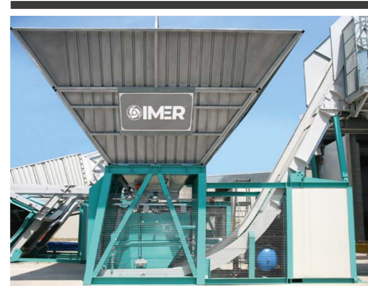
Aggregate storage ONEDAY with weighing skip
