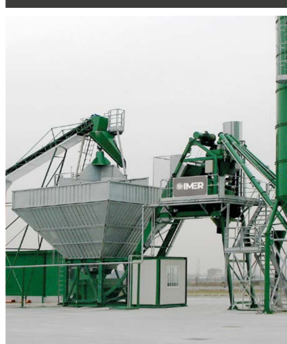
ORU ONEDAY concrete batching plant with aggregate storage, control cabin and incorporated weighing skip.
