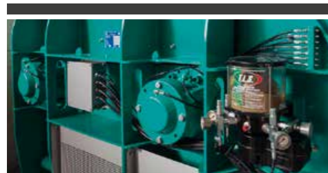
Automatic lubrication system equipped with 4 programmable and independent pumps
