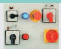
Essential electrical panel with rotation direction selector, double speed selector of the eccentric screw and missing grid warning light and power line presence.
