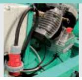
C310 piston compressor, integrated and protected under the cover. Electrically excludable via On / Off button, when not needed.
